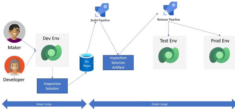
When you export a solution from Dataverse, it's exported as a single compressed file. To store the low-code resources in version control, you could use the build tooling to unpack the solution file into individual component files. During build automation, the build tools combine individual files from version control into a single compressed file.
