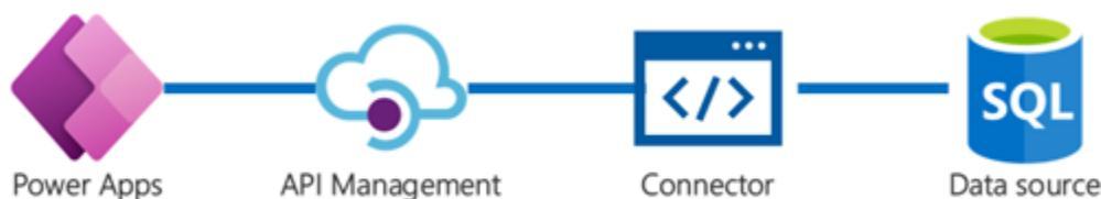
The same architecture is used for all connectors, including custom connectors that you create for your own APIs. The use of Azure API Management ensures a consistent interface for Power Platform products like Power Apps and Power Automate with all connectors.
